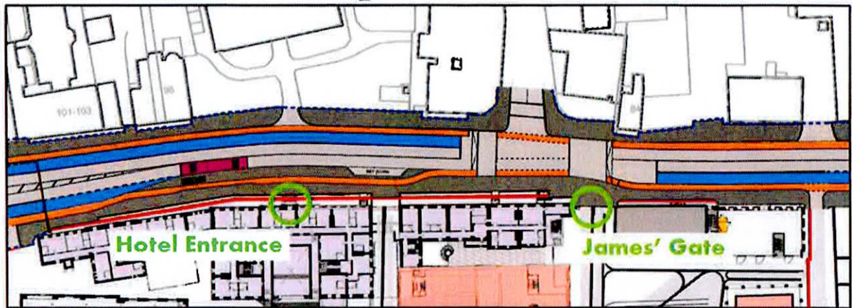
Image 7 – Required local changes to BusConnects layout, showing increased pedestrian space, hotel layby, and relocated bus stop
